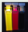
From left to right: saturated solutions of 5, 8 and P1 in Chloroform, in the dark, excited at 380 nm
