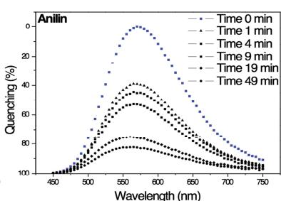
PL quenching experiments with P4 pellets and *p*-toluidine or aniline as analytes.
