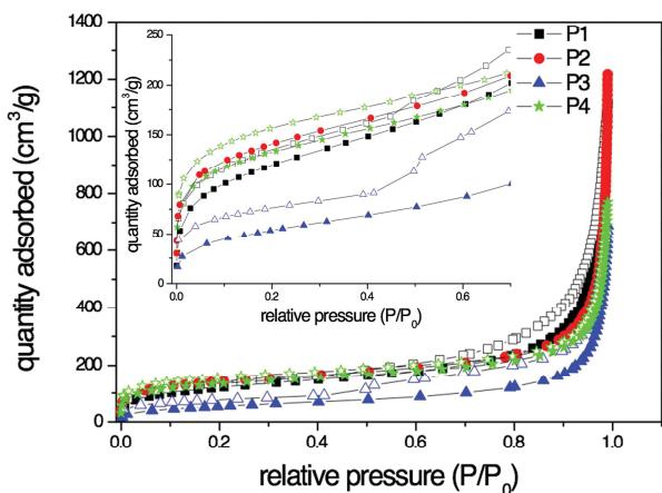
Nitrogen adsorption (filled symbols)/desorption (open symbols) isotherms at 77 K for P1 (black squares), P2 (red circles), P3 (blue triangles), P4 (green stars); the inset shows the pressure range  $P/P_0$  from 0 to 0.7.
