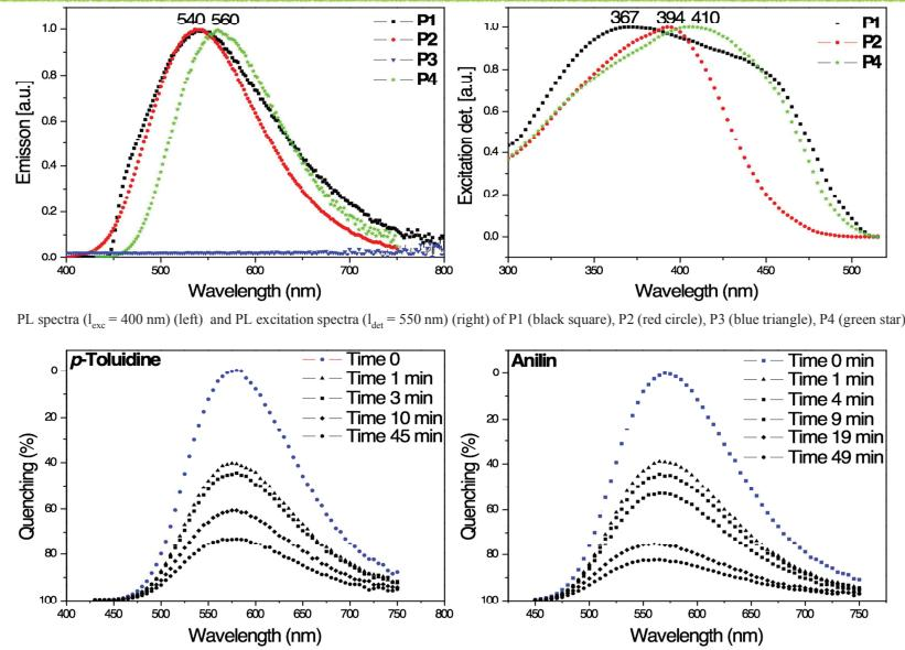
PL spectra ( $I_{exc} = 400$  nm) (left) and PL excitation spectra ( $I_{det} = 550$  nm) (right) of P1 (black square), P2 (red circle), P3 (blue triangle), P4 (green star).
