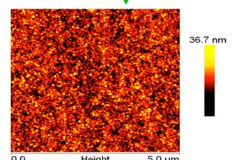
• Contact-mode AFM surface image of a thin film of PCBPBT on ITO (topology).
