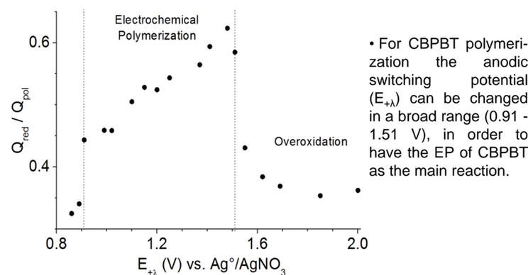
Fig 3. Dependence of the ratio of reduction ( $Q_{red}$ ) and polymerization charge ( $Q_{pol}$ ) on the value of anodic switching potential ( $E_{+X}$ ) that is applied in the first cycle during EP of CBPBT.
