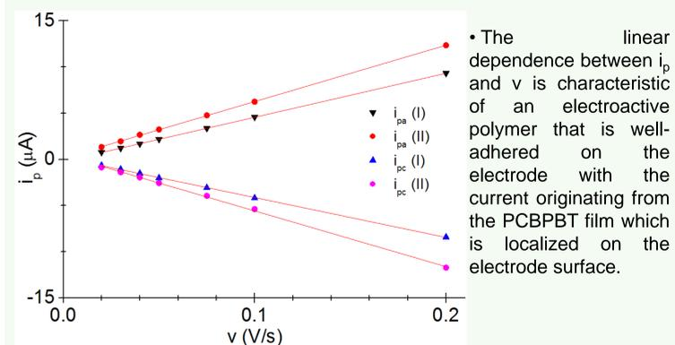
Fig 5. Dependence of the anodic and cathodic current peaks ( $i_{pa}$  and  $i_{pc}$ ) on the sweeping rate ( $v$ ) for a PCBPBT film on ITO in a monomer-free sol. The potential range was 0 - 1 V.
