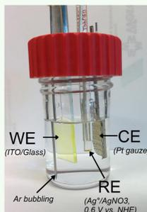
Fig 3. Three-electrodes cell used by us for EP.
