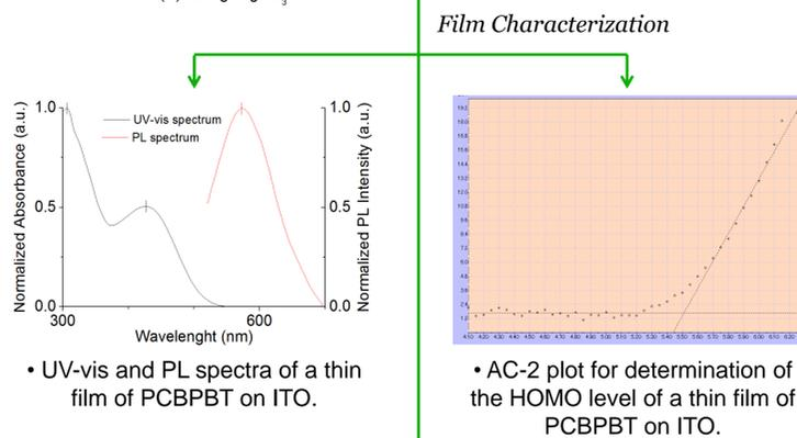
• UV-vis and PL spectra of a thin film of PCBPBT on ITO.
