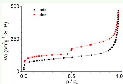
Fig 2. N<sub>2</sub> isotherm of PCBPBT at 77 K. PCBPBT was obtained as a bulk polymer via oxidative coupling (*vide infra*).
