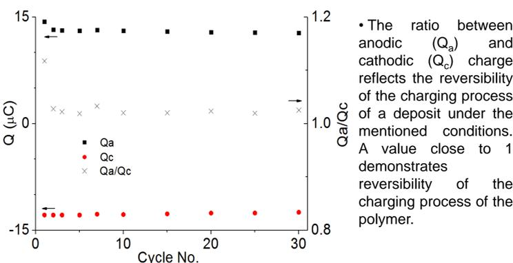
Fig 4. Relationship of anodic and cathodic charge ( $Q_a$  and  $Q_c$ ) and the number of cycles for a PCBPBT film on ITO in a monomer-free sol. The applied potential range was 0 - 0.8 V with a sweeping rate of 0.1 V/s.
